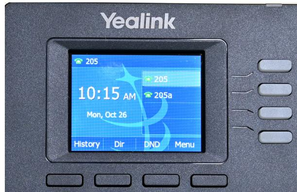
The keys to the right of the screen are programmable Line Keys. Each can be set per the configuration of the phone and/or configured as speed dials or 'favorites'. In the example above, there are two line keys that have been configured on the top two buttons.
