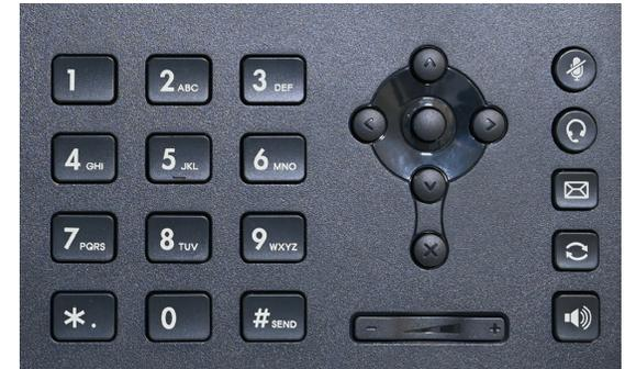
The four-way navigation pad allows the user to move through the phone's menu system and make selections, and the four arrow keys also double as shortcuts. Pressing UP displays the call history, pressing DOWN displays the number directory, LEFT and RIGHT select the line appearance key to use for making an outgoing call.
