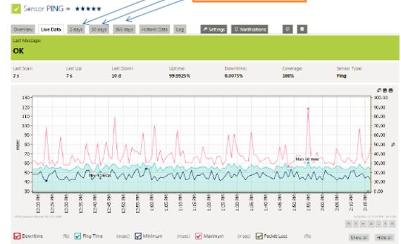
PING Sensor sends packets every 60 seconds to router and plots out several metrics like downtime, ping time (latency), and packet loss. BCN stores up to 90 days of data that can be viewed in a clear, intuitive portal.
