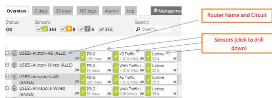
All customer locations along with Router Name and Circuit ID allows a quick view to sensor status.
